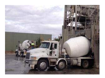
**Step 2:** Add 80% to 90% of the mix water and allow the Helix to mix in the water for **not less than** 45 seconds.
