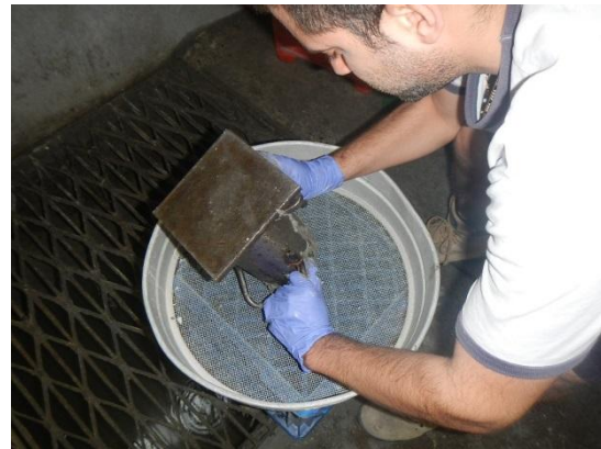
Concrete tipped in tray
