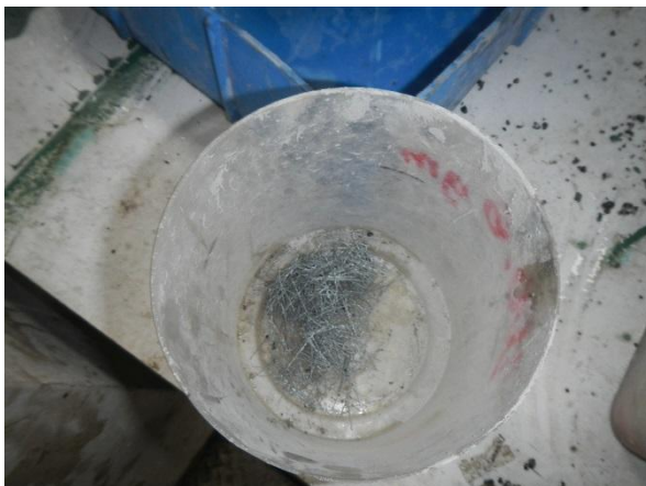
Helix TSMR weighed on scale. Total weight = 41.0
