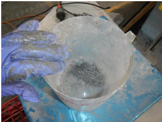
Helix TSMR weighed on scale. Total weight equals 248.2g-200.6g equates to 47.5g
