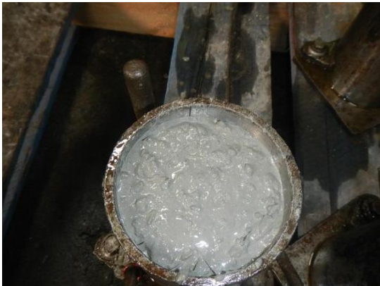
Concrete poured in cylinder
