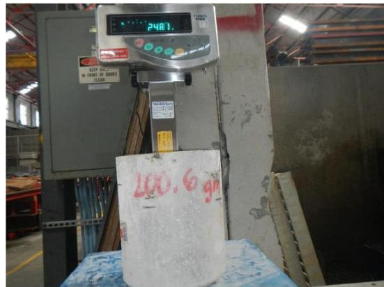
Helix TSMR weighed on scale. Total weight equals 248.2g-200.6g equates to 47.5g
