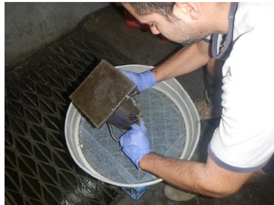
Concrete tipped in tray
