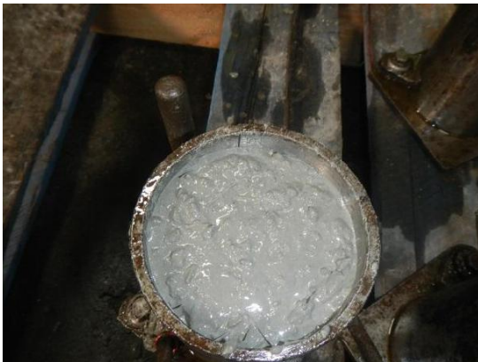
Concrete poured in cylinder
