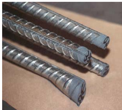
Figure 9. Showing touch-up repair of the cut ends of galvanized rebar using an inorganic zinc-rich paint.
