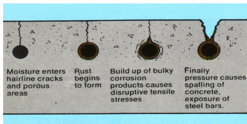
Figure 1. The progress of corrosion-induced damage in concrete.
