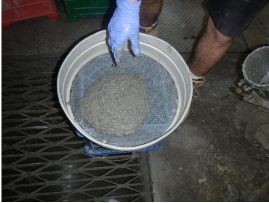
Concrete tipped in tray
