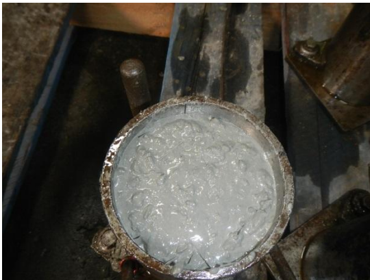
Concrete poured in cylinder
