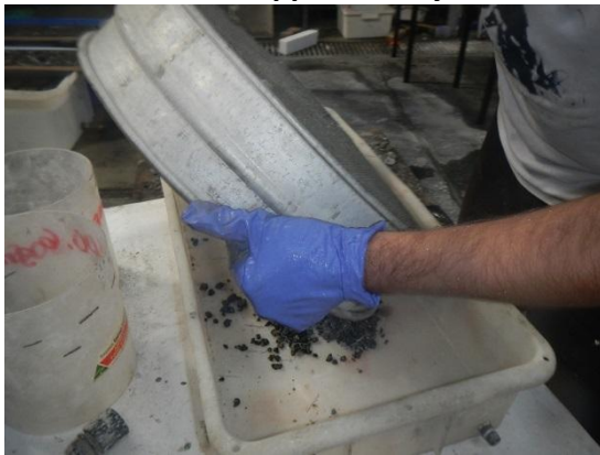
Aggregate and Helix TSMR remain and tipped into tray and Helix TSMR removed with magnet
