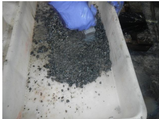
Aggregate and Helix TSMR remain and tipped into tray and Helix TSMR removed with magnet
